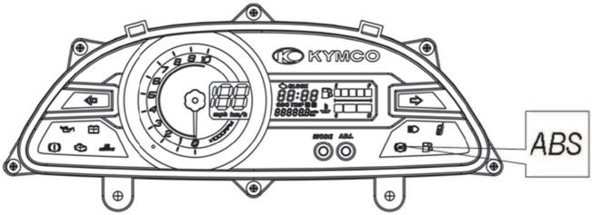
The ABS indicator light is on the right side of the meter. This light will comes on when the ignition switch is turned on and goes off shortly after the vehicle starts moving it stays off as long as the system is ok.
