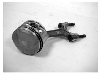
Install the piston and connecting rod into the cylinder with a piston installer.
