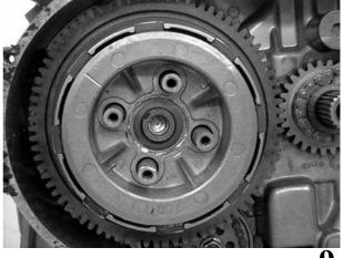
Remove the clutch center, clutch friction disks and plates.
