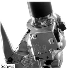
Remove the four upper fork bridge bolts to remove the handlebar.
