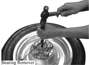
Drive out the wheel bearings and remove the distance collar by using a bearing remover.
