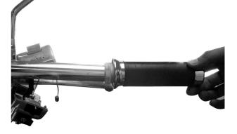
Connect the throttle cable to the throttle grip. Apply grease to the throttle cable. Install the throttle housing by aligning the pin on the housing with the punch hole in the handlebar. Then, tighten the two screws.
