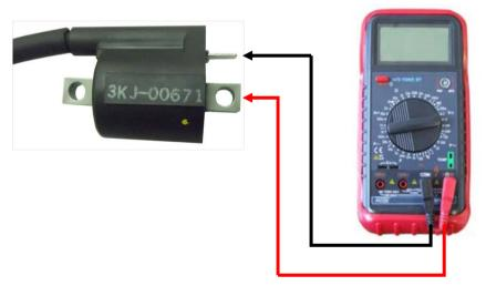
If the values found are incorrect change the coil, erase the error with the OBD reader and run the bike to confirm that the error is complete erase. If the error continues check the point 3.
