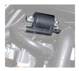
2.- Check the coil resistance, with one multimeter in  $200\Omega$  measure the resistance of the primary circuit (check picture), the resistance can be between 0,2 and 1  $\Omega$ .
