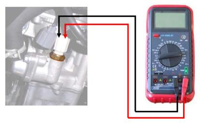
If the multimeter shows short-circuit or open-circuit changes the temperature sensor and erase the OBD error.
