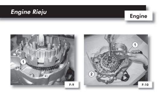
**II) DISENGAGE** the nut from its fixing tab (1/F-9); using the appropriate wrench (1/F-10), unscrew and remove the fixing nut (2/F-10) of the clutch boss.
