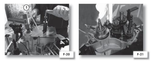
**23) SEPARATE** the 2 crankcases by gentling tapping the secondary shaft and shift shaft with a wooden mallet.
