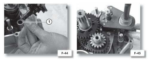
5) FIT the countershaft in the clutch crankcase. *N.B.: assembly of the countershaft in its seat implies no interference.*
