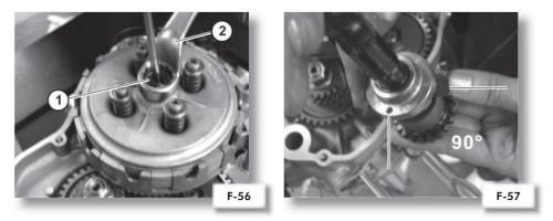
**21) FIT**: the dowel bolts and a new gasket on the crankcase; the clutch cover; if necessary, this operation can be made easier by turning the impeller of the water pump. Secure in place with screws (**Cs**  $1.0 \div 1.2 \text{ kg}^*\text{m}$ ).
