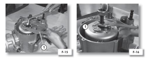
**17) REMOVE** the rotor of the magneto flywheel by means of the appropriate puller (I/F-16), which must be screwed into the threaded seat of the rotor; whilst holding the latter in place with a wrench, turn the centre screw.
