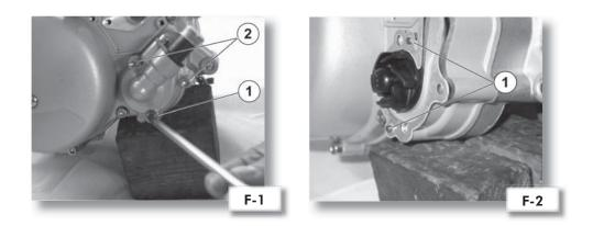
**3) UNDO** the fixing screws of the flywheel cover (left hand side) and remove it. Remove the starter motor (if fitted) by removing the two screws on the crankcase and the screw on the support strap.
