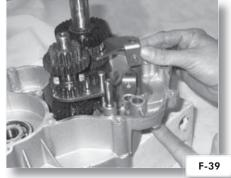
**3) FIT** the desmodronic shaft (F-40). Insert the fork guide pins into the desmodronic shaft (F-41).
