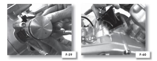
**23)** In the order indicated, FIT the piston rings, making sure that the ends are correctly positioned in the seats on the piston; a new cylinder gasket; the cylinder; the centre cylinder O-ring in the stud bolts; the O-ring on the cylinder head; the head (clean beforehand). Tighten the nuts evenly and diametrically (**Cs**  $1.4 \div 1.6 \text{ kg}*\text{m}$ ); check the position and tightness of the O-ring on the cylinder head.
