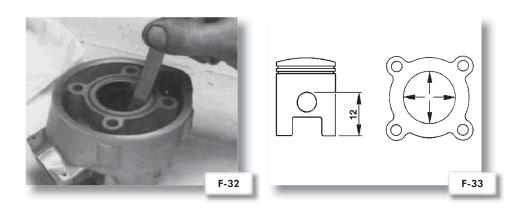
Repeat the measurements in several positions along the cylinder jacket, between the top face of the cylinder and the exhaust gap (F-34).
