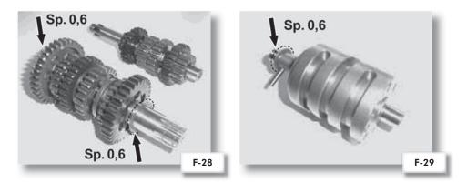
**5) CHECK** the distance of the shim washers of the shift shaft both on the crankcase and on the part, and fill any gaps with other shim washers, as shown in the photo (F-30). The end float must be less than 0.1 mm.
