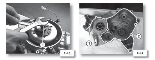
**8)** FIT the 13 fixing screws and tighten in place (Cs  $1.0 \div 1.2 \text{ kg}^*\text{m}$ ). Make sure all shafts can turn freely. Make sure that none of the shafts feature excessive end play, in which case, separate the crankcases and replace the top shim washer with another having a more suitable thickness.
