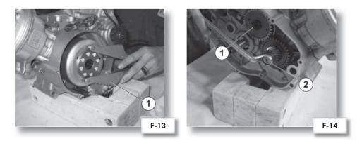
**15) UNSCREW** the nut (2/F-14) with a 19 mm wrench, whilst holding the flywheel in place with the special wrench; then remove the following parts in this order: drive pinion, countershaft drive gear, key, spacer bushing and O-ring.
