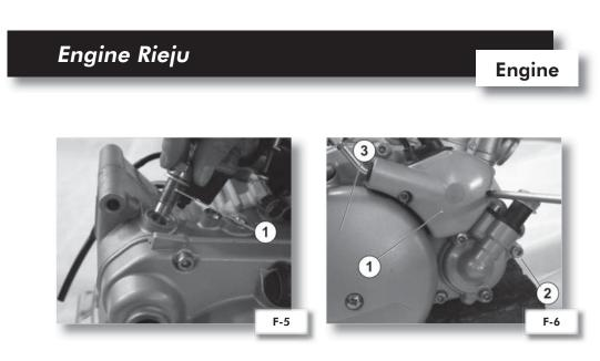
6) **REMOVE** the sliding stop screw for starting from clutch side (I/F-5).
