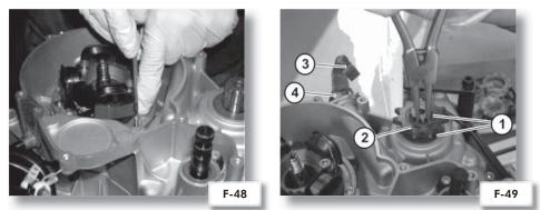
12) CHECK operation of the sprocket and gear wheel pair.
